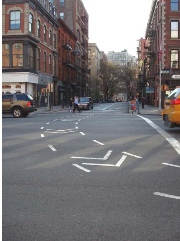
Figure 23: Many intersections in New York have markings to guide cyclists through to facilities on the other side, such as here in Manhattan, where Bleeker Street crosses The Bowery.
