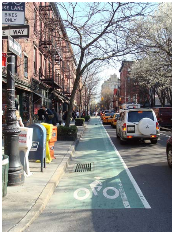
Figure 21: This green bike lane on Bleeker Street in Greenwich Village provides much less protection than a buffered bike lane or cycle track, but at least it is clearly marked.
