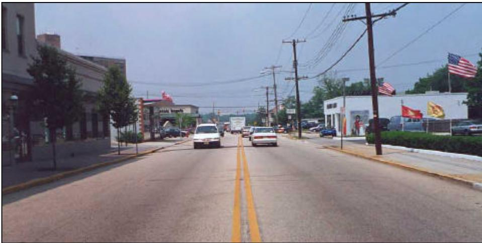
***Picture 2.1-7: Although mixed retail/ commercial land use, this state highway is poorly designed for pedestrians. Wide lanes and no place to cross. Red Bank, NJ.***
