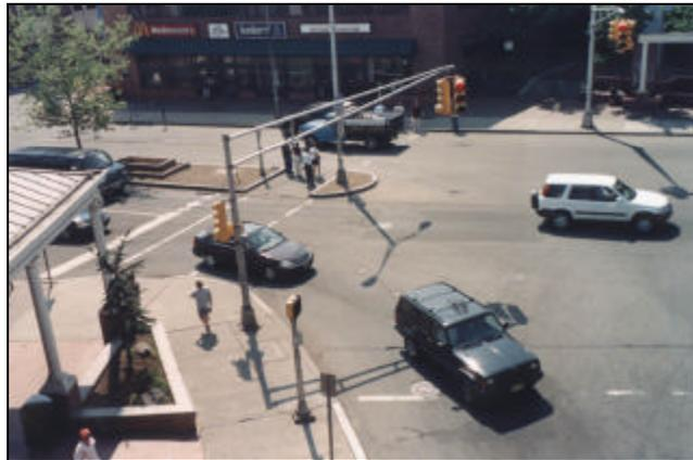
***Picture 2.1-2: Wide turning radii - with the primary purpose to accommodate trucks and buses - allows motorists to make a fast turn and as a result puts pedestrians at risk at this downtown intersection. New Brunswick, NJ.***
