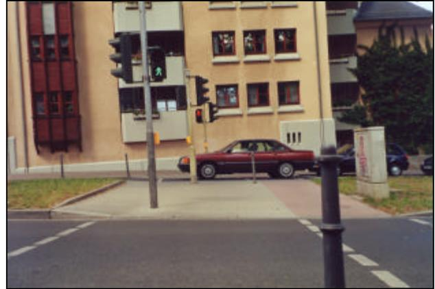
*Picture 3.4-1: A crosswalk, nice wide median and two-phase push-button signal with almost immediate response ensures a safe and convenient crossing for pedestrians (and cyclists). Germany.*
