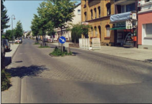
**Picture 3.2-1: Cobblestone surface texture and tree planted islands to reduce motor vehicle speeds. Germany.**
