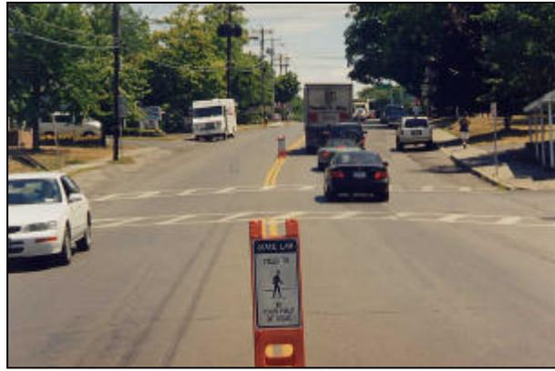
**Picture 2.3-4: Marked crosswalk at unsignalized intersection with post-mounted pedestrian warning signs – New Paltz, NY.**
