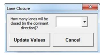
**Step 5.1**: Enter the number of lanes to be closed in the dominant direction. The maximum number of lanes that can be closed is one less than the total number of lanes in the work zone. If all of the lanes are to be closed, this would be classified as a Road Closure.
