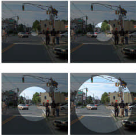
Figure 8.9: Fields of Vision at 30, 25, 20 and 15 mph Respectively
