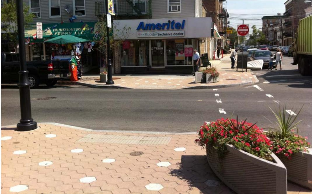
Figure B3 – Monroe St & Ferry St – Greatly improved sidewalk aesthetic quality and planters along Ferry Street. Curb bump outs make crossing safer, but intersection is still uncontrolled.
