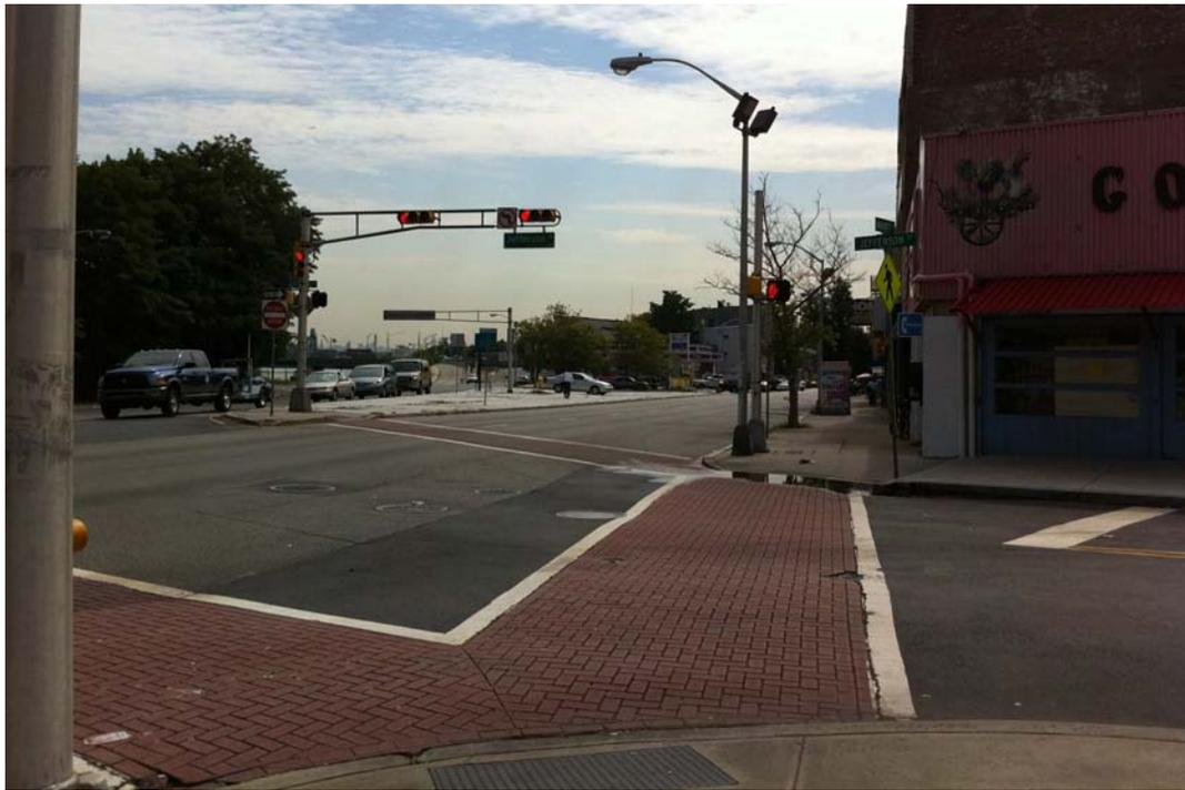
Figure B1 – Improvements along Market Street consist of mainly striping, ADA sidewalk ramps, and pedestrian crossing signs.
