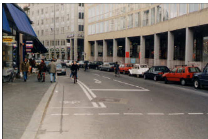
Picture 65: Staggered Stop Lines, Munich, Germany (MK)
