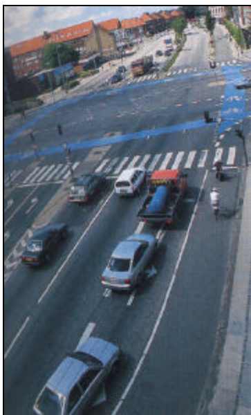
Picture 11: Blue bike lane crossings marked through intersection. Note: Cyclists get a head start due to recessed stop line for motor vehicles in right-turn lane. (DK)
