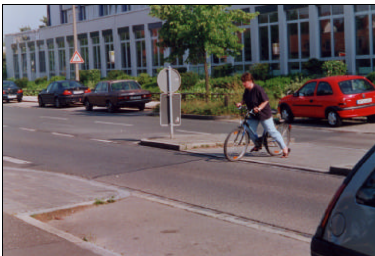
Picture 29: Refuge Island/ Median) at unsignalized crossing. (MK)
