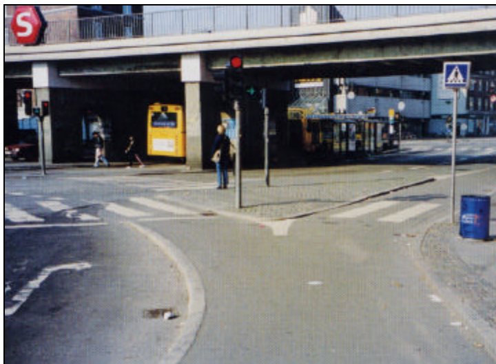
Picture 68: Pre-right-turn for cyclists to avoid signal, but not pedestrians (DK)
