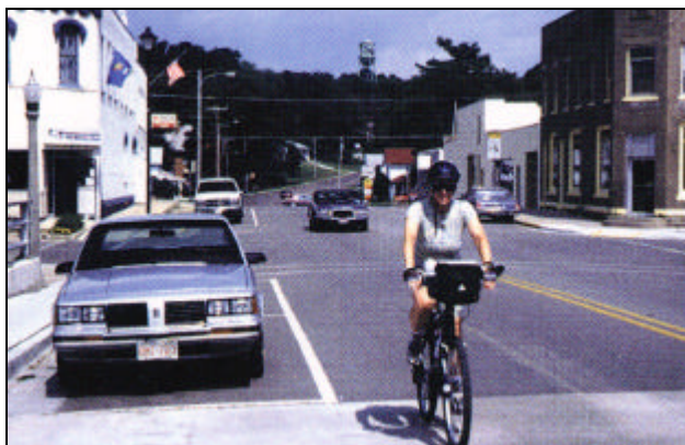
Picture 1: Wide outside lane with parking. Source: AASHTO.
