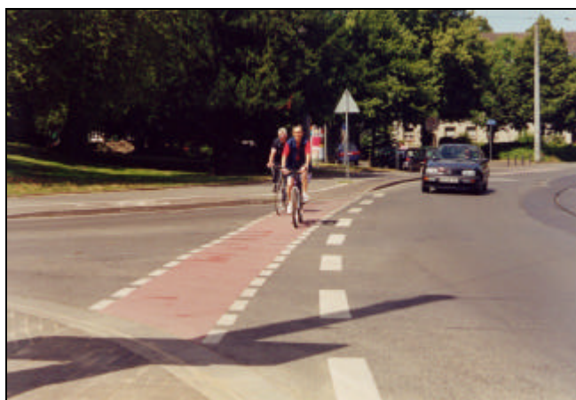
Picture 15: Cycle track continued as colored lane through intersection. (MK)
