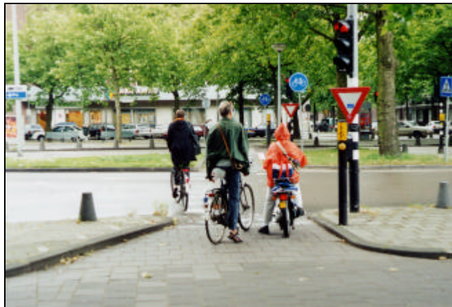
Picture 13: Separate cycle facility at signalized intersection, The Netherlands. (PS)
