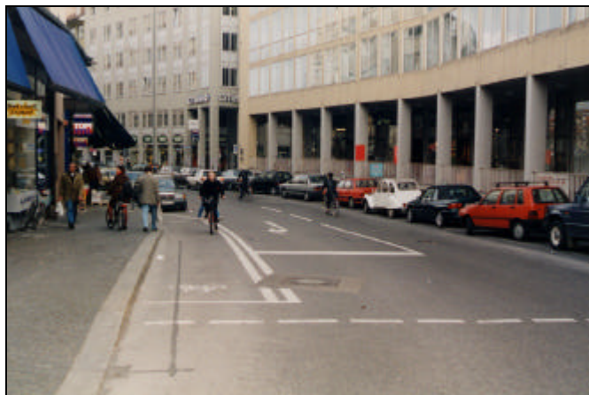
Picture 27: Staggered Stop Lines, Munich, Germany. (MK)
