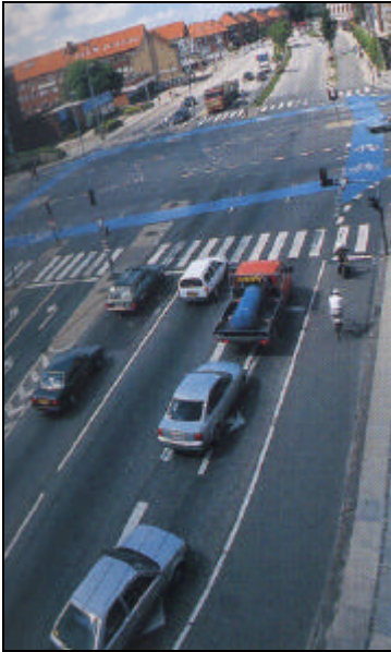
Picture 56: Blue bike lane crossing marked through intersection (DK)
