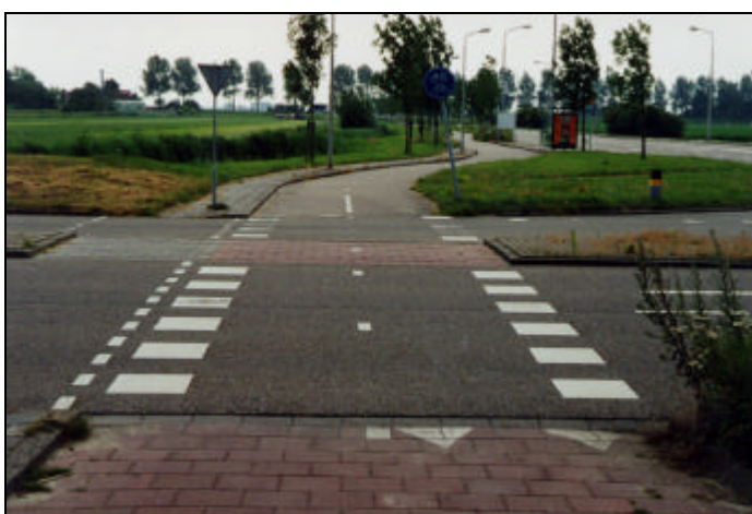
Picture 61: Bend-out cycle track (suburb of Amsterdam) (PS)
