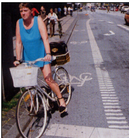
Picture 20: Cycle track becomes broken bike lane before intersection with right-turn motor vehicle lane.
