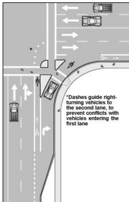
Figure 6: Bike lane through dual right-turn lanes with island.
