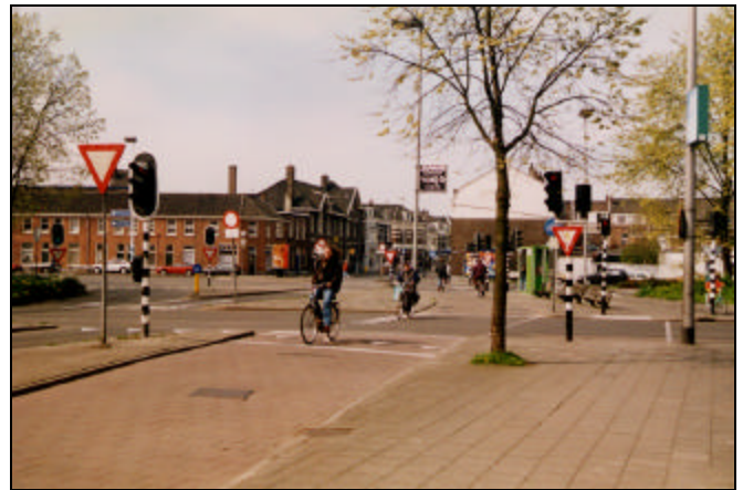
Picture 59: Separate cycle facility at signalized intersection, Germany (MK)
