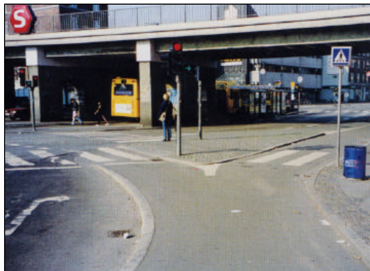
Picture 24: Pre-right-turn for cyclists to avoid signal, but not pedestrians. (DK)
