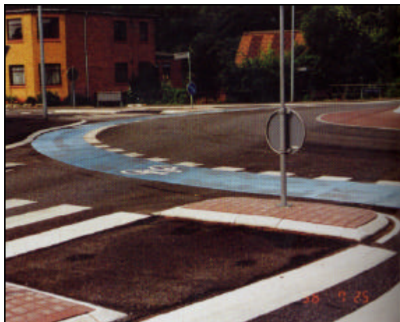
Picture 74: Blue bike lane an option in roundabouts (MK)
