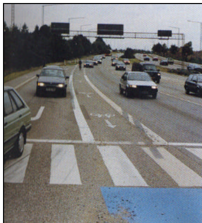
Picture 62: Merge with right-turning vehicles long before the intersection (DK)
