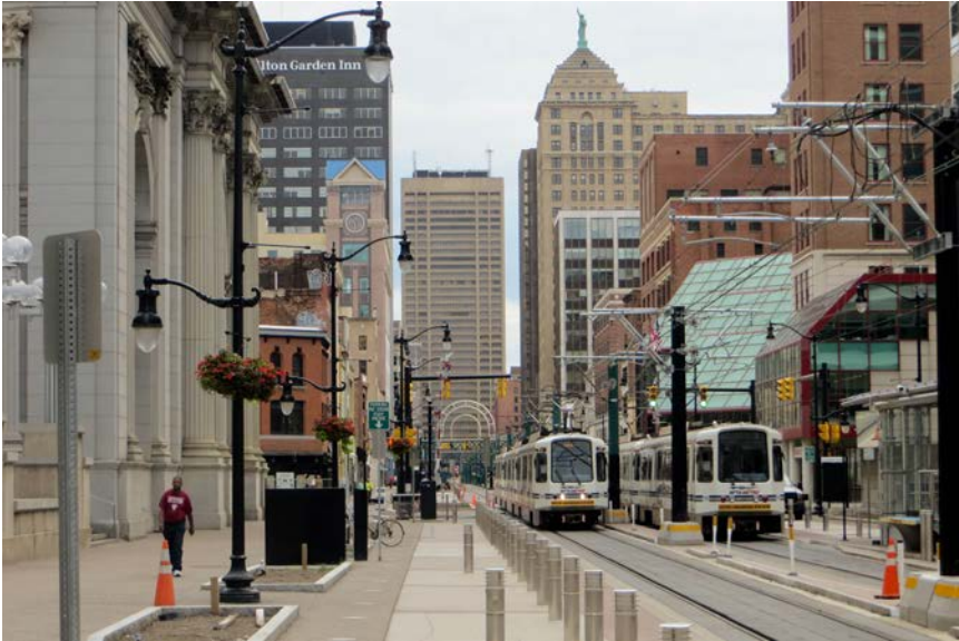
The Niagara Frontier Transportation Authority (NFTA) originally envisioned an 11-mile “heavy rail” system for Buffalo, akin to the Washington, DC Metro. AMV helped NFTA convert the plan into a light rail that runs 6.4 miles along Main Street. It began operating in 1984. Image: David Wilson, Wikimedia Commons
